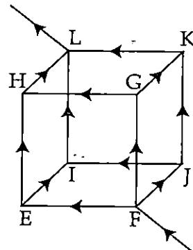
A current of  $2A$  is sent in at the vertex F and a current of  $2A$  is drawn out at the vertex L. The arrows show the direction of the current at each edge. The current through the edge JI is :
